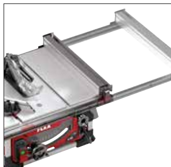
High-precision parallel fence with rack and pinion system. Supports longitudinal cuts up to 427 mm on the left side and 780 mm on the right side. Very smooth and quick adjustment
